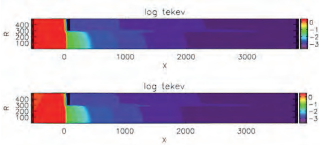
Figure 116: Electron temperature distributions in the CRASH target at the time 0.9 ns. Top panel: the output from the standard version of the CRASH code (no NLTE effects). Bottom panel: the coupled CRASH-RADIOM code, with E_{\text{rad}}/B set to 1 in the data passed to RADIOM. There is a slight difference in color scale, reflecting the behavior in the laser corona discussed in the text.
