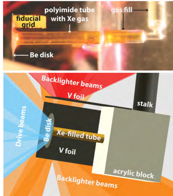
Figure 13: A photograph (top) and model showing laser the interaction of laser beams (bottom) with a target used to create a radiative shock in laboratory experiments. A Be disk behaves as a piston to shock and compress Xe gas in a polyimide tube. The tube and target stalk are inserted into an acrylic block. Two V foils are attached to the target to create x-rays to enable observation of the shocked Xe.
